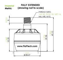
The height of the Equalizer reduces as it compresses when installed under the table.
